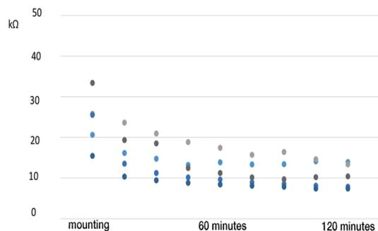
**Fig 5. Sequential change of impedance of new electrode on scalp without shaving or degreasing.**
