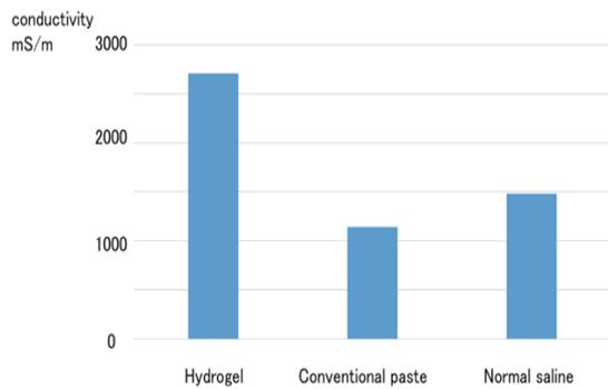
**Fig 2. Conductivity of hydrogel, conventional EEG paste and normal saline (mS/m).**
