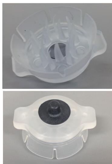
**Fig 1. Prototype of Kenzan shaped electrode made of hyper conductive elastomer.**
