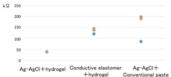
**Fig 4. Impedance of the candidate combination of electrode tip and gel ( $k\Omega$ ).**
